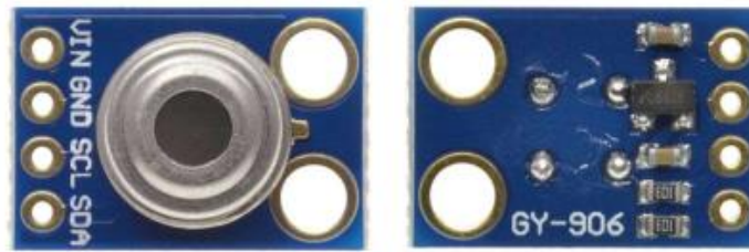
Figure 3. MLX-90614 temperature sensor integrated into the GY-904 module.
