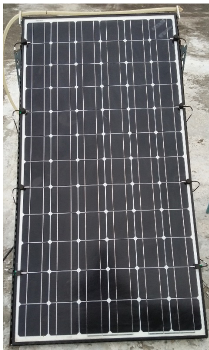
Fig. 4. Photovoltaic panel with temperature sensors
