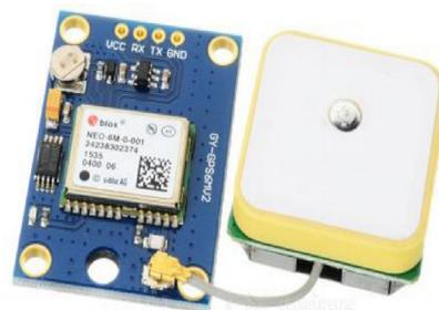
Gambar 4: Modul GPS Neo 6v M2
