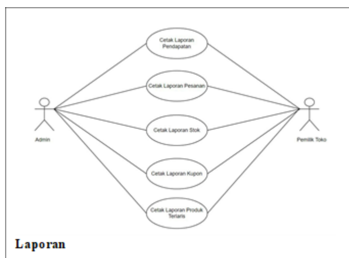
Gambar 8. Use Case Diagram Laporan
