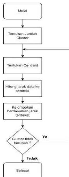
Gambar 4 Diagram Alir K-Means Clustering
