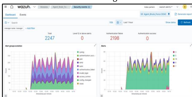
Figure 18 Authentication Failure Brute Force Attack (1 Hour)
