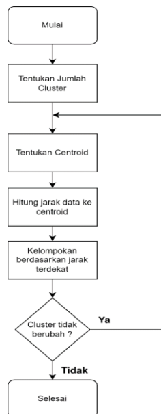
Gambar 4 Diagram Alir K-Means Clustering
