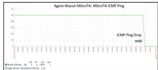
Figure 24 ICMP ping loss attack DoS
