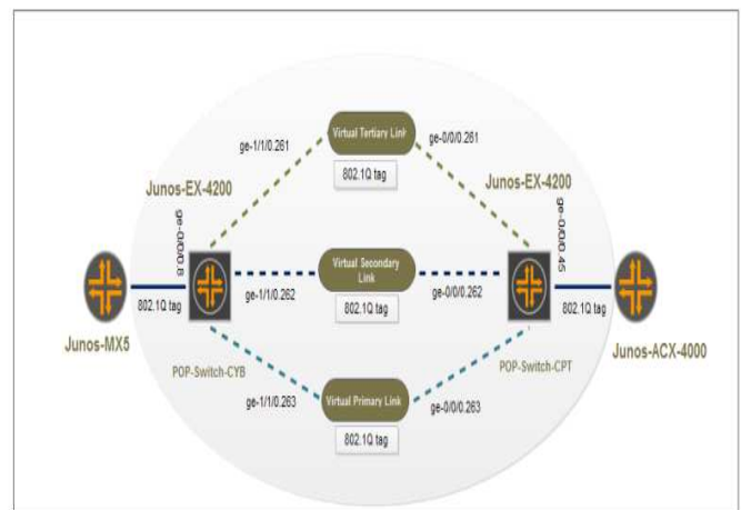
Figure. 4. Schematic and Modeling of 802.1Q tags in a Metro-Ethernet Multipath Environment
