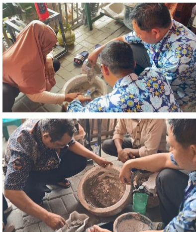
Figure 7. Paving block mixture making process
