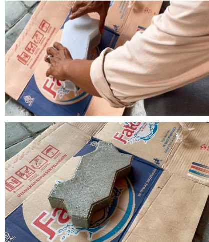
Figure 8. Paving Block Printing Process
